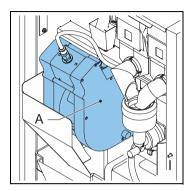
The brewer (A) receives the product from the grinder. The product is made after adding pressurized hot water. The brewer transfers the product to the outlet and transfers the residue to the waste bin.
