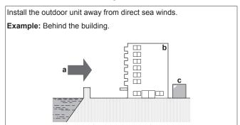
If the outdoor unit is exposed to direct sea winds, install a windbreaker.
