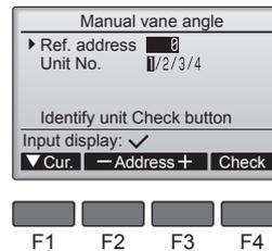
① First, confirm by setting "Ref. address" to 0 and "Unit No." to 1.
