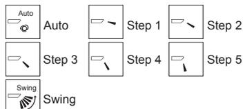
Select "Swing" to move the vanes up and down automatically. When set to "Step 1" through "Step 5", the vane will be fixed at the selected angle.
