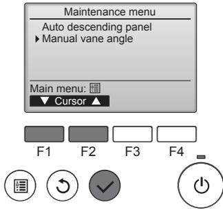
② Select "Manual vane angle" with the [F1] or [F2] button, and press the [SELECT] button.
