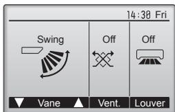
Press the [F1] or [F2] button to go through the vane setting options: "Auto", "Step 1", "Step 2", "Step 3", "Step 4", "Step 5" and "Swing". Select the desired setting.
