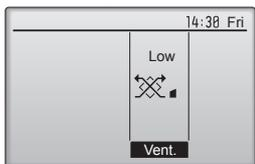
Press the [F3] button to go through the ventilation setting options in the order of "Off", "Low", and "High".
