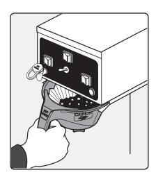
4 Slide the filled brew basket into the brew rails under the control panel. Slide it all the way back until it stops.
