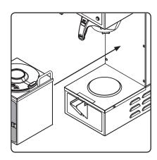
2 Place an empty satellite under the brew basket. Push it all the way back against the front cover. Press the WARMER button to preheat the satellite.
